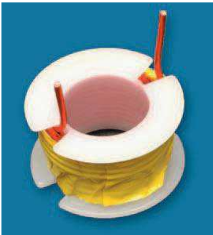
Here's what a completed inductor looks like (you need two), prior to scraping off the enamel insulation and tinning the leads.
